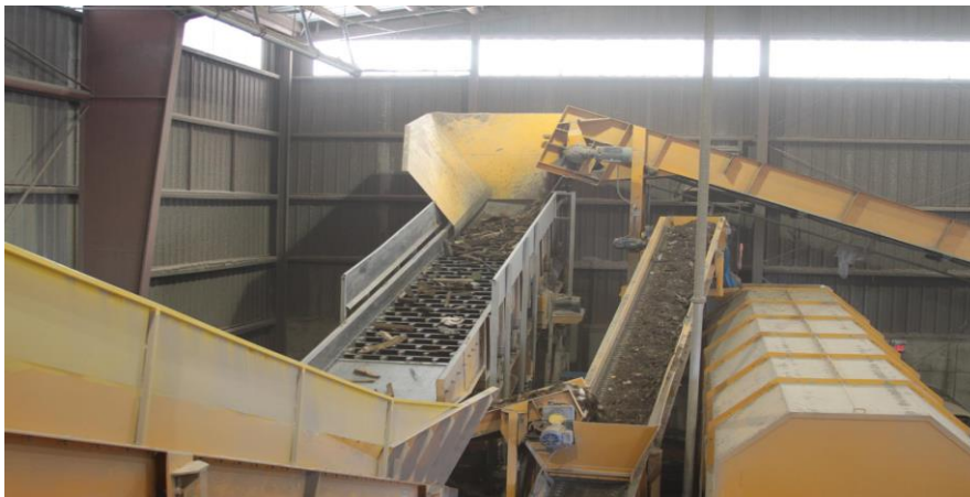
Figure 23. As the debris is carried upon the conveyor, it is placed on top of a series of screens.
