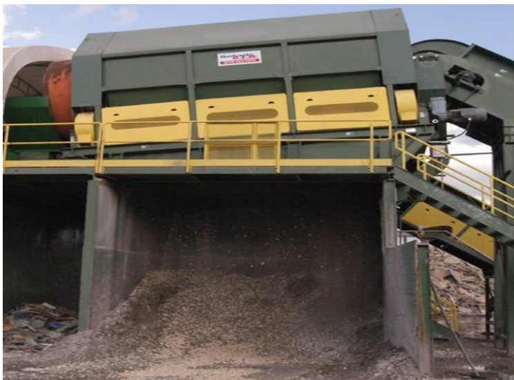
Figure 24. The debris that falls through the screens is collected as recovered screened material or fines.
