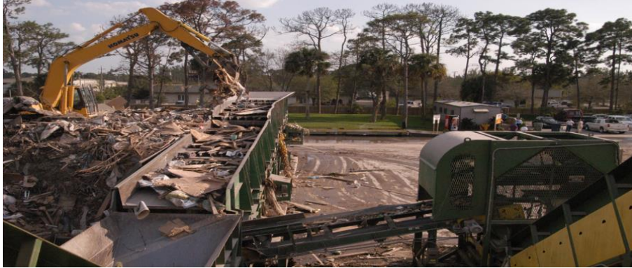
Figure 22. Start of facility where the debris is placed on the conveyor belt to be sorted using manual and mechanical measures.
