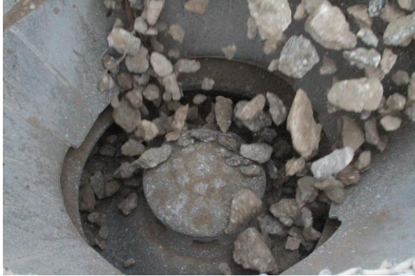
Figure 29. Crushed concrete is commonly used as a replacement for construction aggregate
