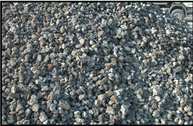
Crushed concrete is commonly used as a replacement for construction aggregate
