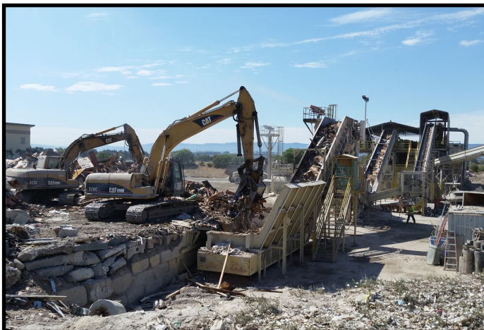
CDRA members use a combination of mechanical equipment and trained employees to separate debris from construction, demolition and renovation projects into marketable commodities
