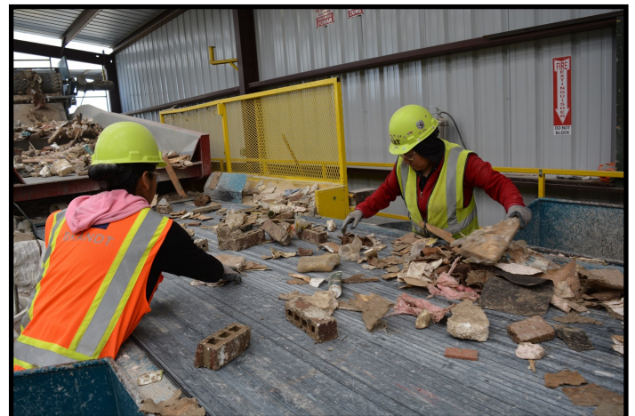
CDRA members use a combination of mechanical equipment and trained employees to separate debris from construction, demolition and renovation projects into marketable commodities
